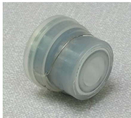
Figure 2 - Oxygen cell showing thermistor
